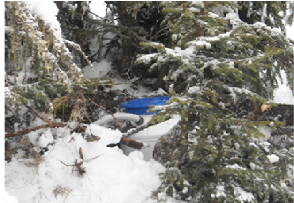
Figure 3. The infrasonic sensor partially covered by snow in early winter 2012/13 (photo: G. Ulivieri).
