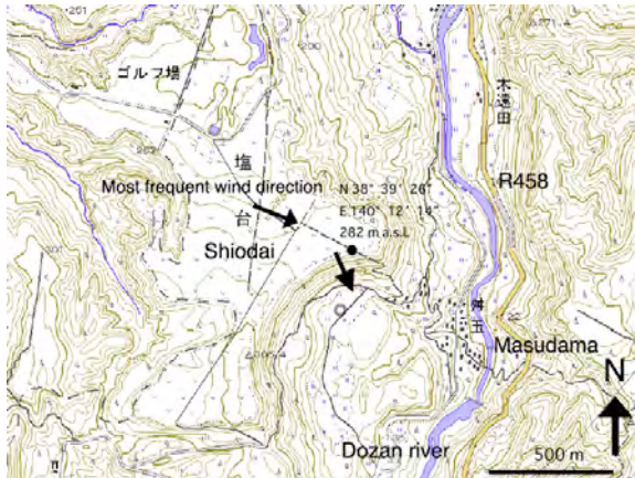
Figure 2. Topographical map around the test site. A short arrow on the slope means the main avalanche pass, a long arrow on the plain the most frequent wind direction. ●: AWS installed at the leeward end of the plain, ⊙: Web camera at the bottom.
