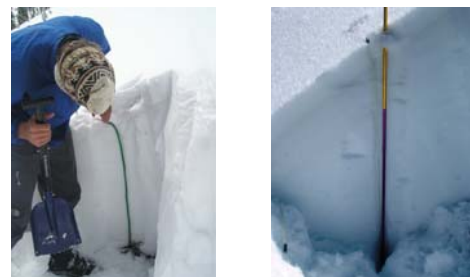
Figure 3. Vertical boreholes were used to document snowpack deformation during April of 2004. Holes were placed in groups of three, 1 meter apart, and perpendicular to the fall-line of a 30-degree slope. They were set using a vertical avalanche probe and filled with 8mm nylon utility cord. Boreholes were placed April 13th, and excavated April 16th, 19th, and 23rd. Deformation was determined by aligning a vertical probe with the ground-borehole interface and measuring the perpendicular distance from the probe to the center of the 8mm cord.
