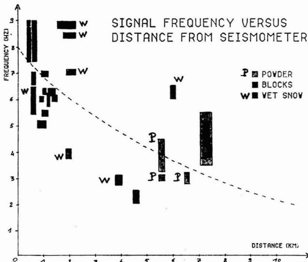
Figure 5. A rectangle was plotted for every avalanche whose distance and frequency were known. Rectangle size describes frequency range and distance range between top and bottom of avalanche path. The dashed line is an exponential decrease shown as a comparison:  $f = f_0 \exp(-k d)$  with  $f_0 = 8\text{Hz}$   $k=0.13 (\text{km})^{-1}$ . The wide range of frequency obtained for a given distance is a result of various conditions regarding snow-type, slope, and position of sliding surface .
