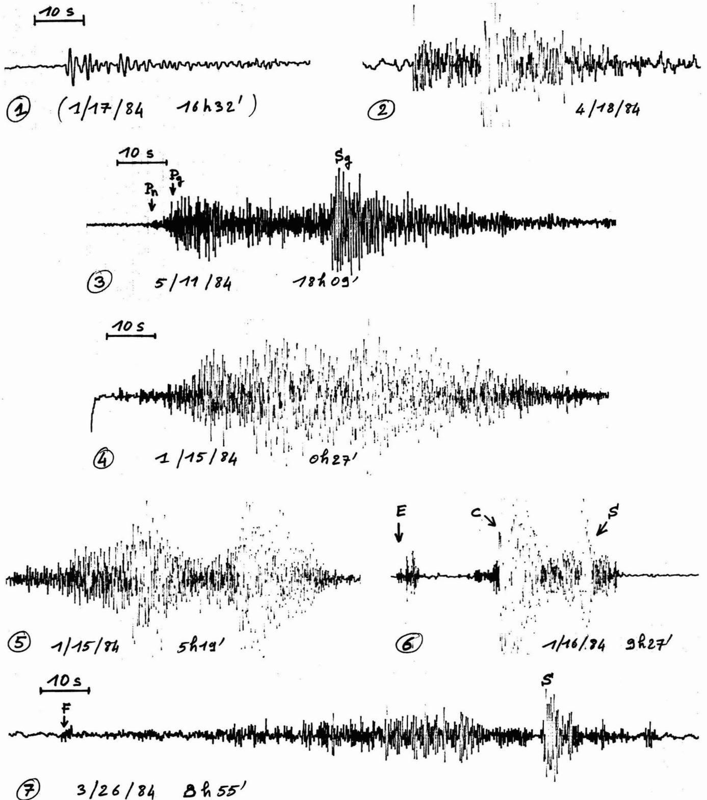
Figure 3. Various kinds of seismic and avalanche signals . 1=distant earthquake ; 2=Mine shot (110 Km) ; 3= local earthquake (270 km) ; 4 and 5= powder snow avalanches ; 6= artificial released avalanche (1km) , E=explosion, C=jump over a small cliff, S=stop ; 7= slab avalanche released with ski, F=fracture, S=stop .(distance:0.7 km) .
