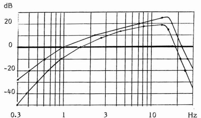
Figure 1. Response curves of the measuring device without (top line) and with (bottom line) output filters. The useful frequency range lies between 2 Hz and 10 Hz . Low frequencies are mainly concerned by far earthquakes and swell-generated natural noise . Frequencies over 10 Hz are disturbed by industrial noise of skilifts and cable-car motors .
