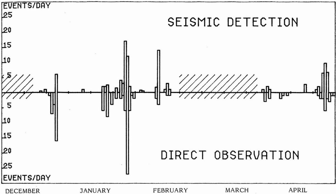
Figure 4 . Daily numbers of detected (upwards) and observed (downwards) avalanches . The artificially released reported to be "small" avalanches were not taken into account . Hatchings were drawn when no data were available because of a lack of observation in early december and recorder failure in march .
