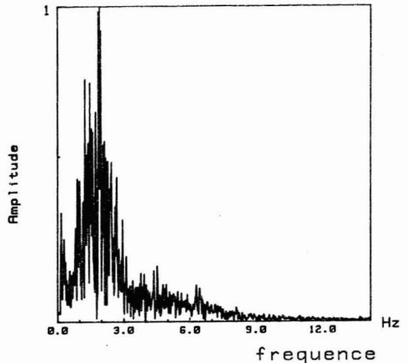
Figure 6. Spectral analysis of two typical signals : Above,powder-snow avalanche of 1/23/84 21h55'. Below, local earthquake of 1/30/84 20h08'.
