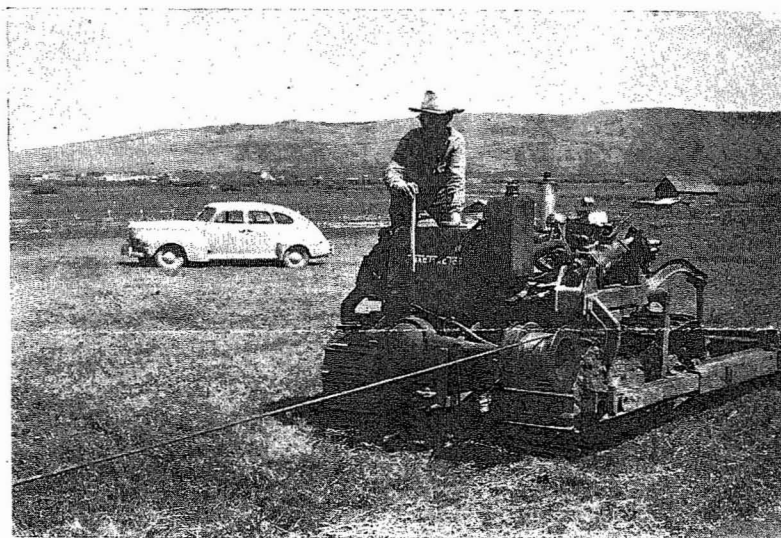
A home made winch attached to a crawler type tractor in Nebraska.
