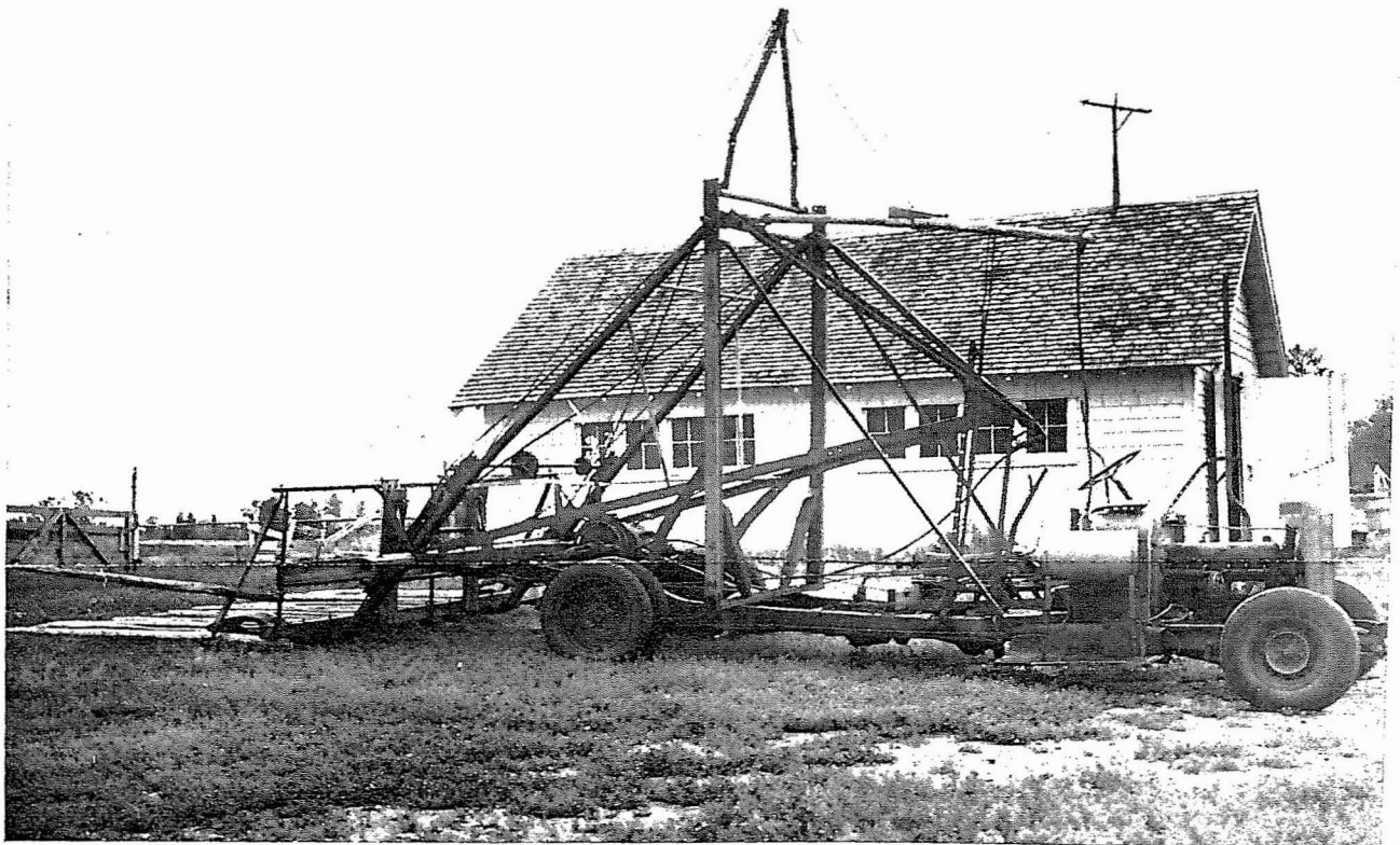
Hay stackers capable of picking up the hay in the field and putting it in the stack are becoming very popular. This one built on an old truck chassis by Wesley Davis near Belgrade, Mont., makes haying considerably faster and easier.
